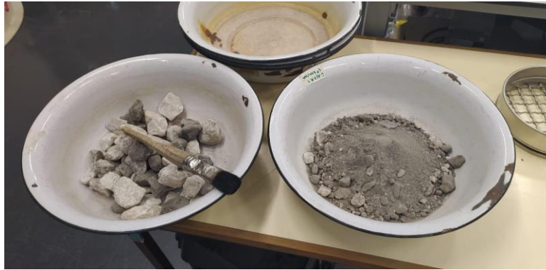
Figure 12: Fines' determination process in the original sample before grinding. On the left there is the coarse greater than 22.4mm and on the right there are the rest of the sizes, still to be separated.
