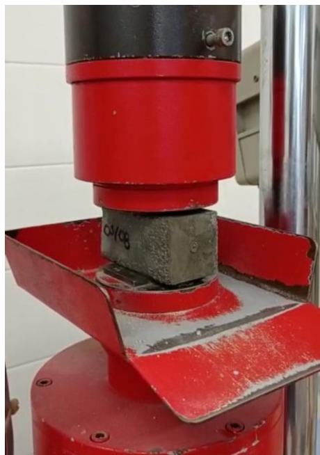
Figure 22: Image of the compression test being carried out.
