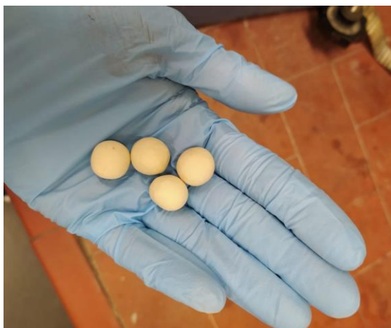
Figure 14: Ceramic balls on top of the screen to decrease the attachment of the particles through the sieves.
